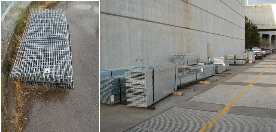
Figure 3: Diffuser gratings in stacks. [Photo credit: Robert Cordie, US Army Corps of Engineers]
