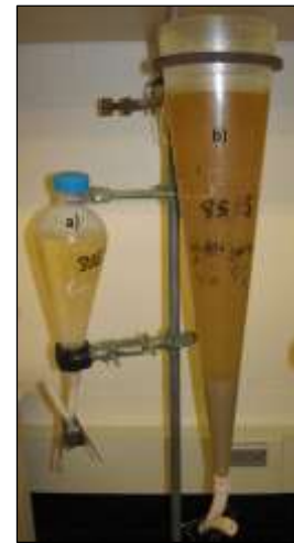
Figure 6: Equipment to concentrate bivalve larvae including a) separation funnels and b) Imhoff settling cones.
