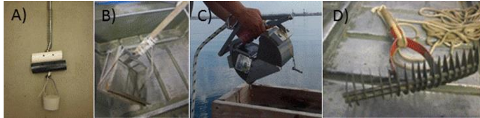
Figure 2: AIS sampling equipment including A) Portland Sampler, B) surface scraper, C) grab sampler, and thatch plant rake.
